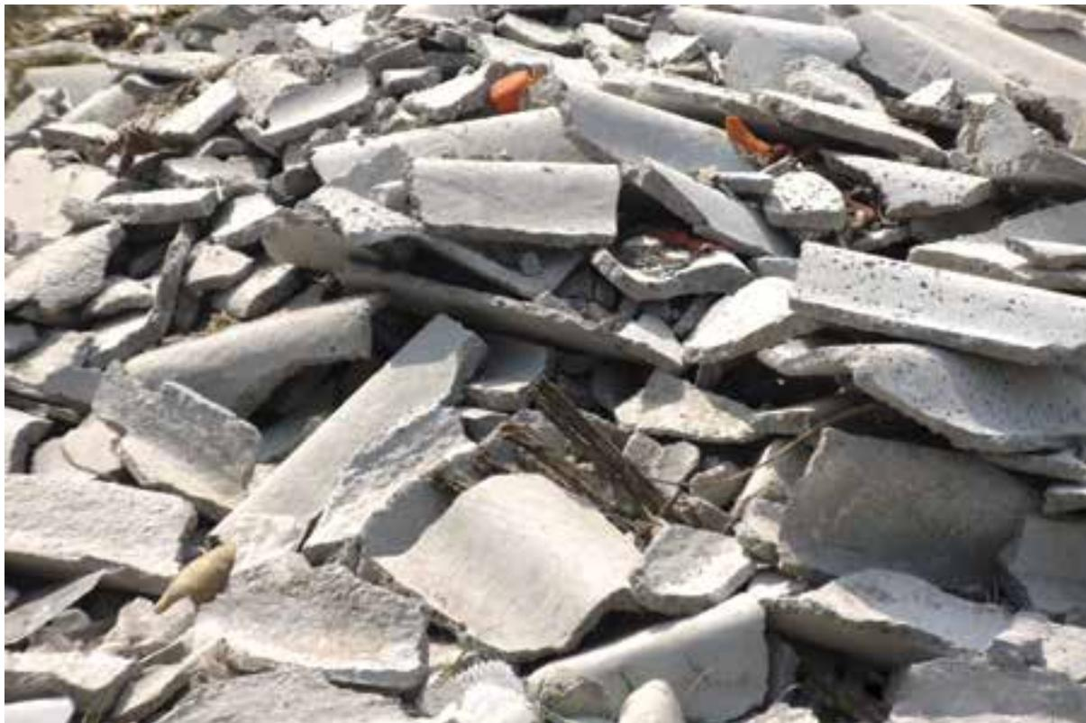
Figure 21. Crumbled corrugated asbestos sheets in Ranigunj, Sharlahi, Nepal
